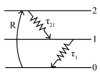
If the pump rate R is  $10^{20}$  atoms cm<sup>-3</sup> s<sup>-1</sup> and the decay routes are as shown with  $\tau_{21} = 20$ ns and  $\tau_1 = 1 \mu s$ , the equilibrium populations of states 2 and 1 are, respectively,
